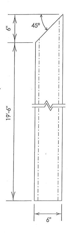
GALVANIZED 6"x6"x 1/2 " TUBING (ASTM A500)
