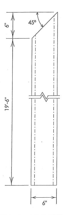
GALVANIZED 6"x6"x 1/2 " TUBING (ASTM A500)
