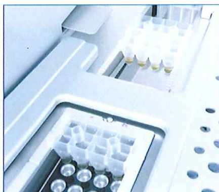
Automated heated lysis and purification from sample volumes of up to 1 ml.
