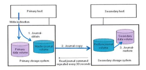
The figure on the previous page illustrates UR software's application of performance optimized, disk-based journaling. In this illustration, online transaction processing (OLTP) data volumes at the primary data center are being replicated to a second VSP at the remote data center.
