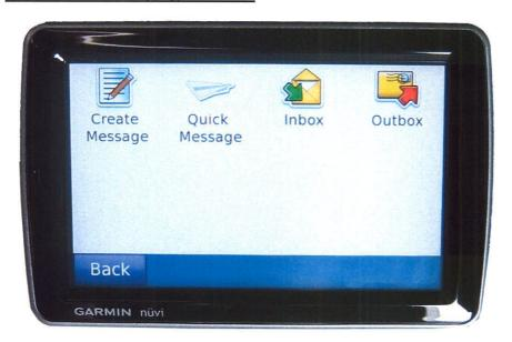
The RSI Garmin Unit can be configured to provide a simple two-way messaging interface between the driver and AVL mapping operator. All messages sent by the driver are time and location tagged and can be used for a variety of status updates and activity reporting.
