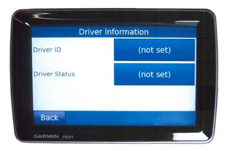
The RSI Garmin Unit allows the driver to log in to a vehicle with a unique ID as well as status.
