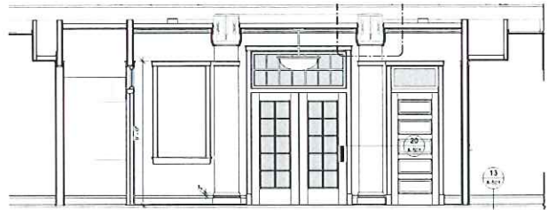
The Reception Area has new trim, ceiling and cornice detailing.
