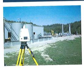
Since March of 2011, Allegheny Surveys has been providing ground-based High Definition Scanning (HDS) services to its clients. Using a Leica C10 ScanStation with Cyclone Software, a highly accurate scan can be made of a large project site in a fraction of the time that it would take field crews to survey it conventionally. Scans can be done in a single day and a detailed topographic map produced quickly and efficiently by exporting the information into AutoCAD.
