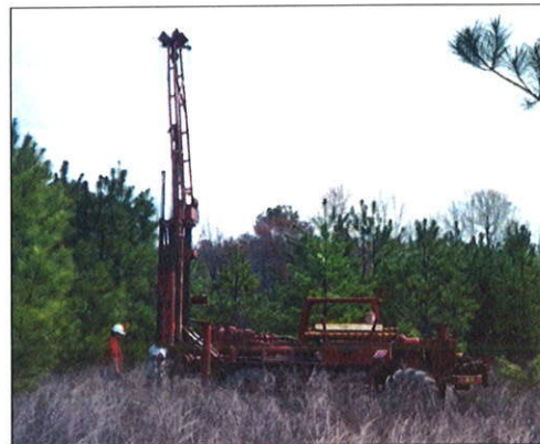
CTL's ATV can drill in rough terrain
