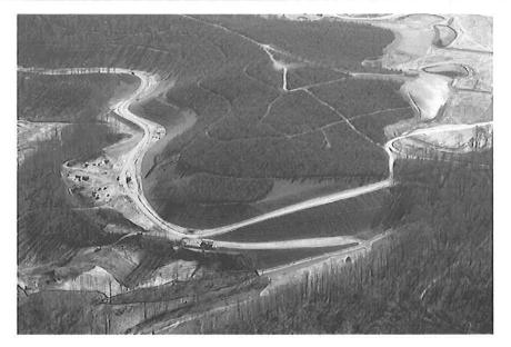
TERRADON has extensive knowledge and experience on all types of AML problem areas. This photo is taken from our Garden Ground Highwalls Project in Fayette County, WV. The photo shows a portion of completed Highwall A on Phase I. The entire project entailed regrading over 14 miles of dangerous highwalls and sealing over 90 portals and will ultimately be utilized by the Boy Scouts of America.
