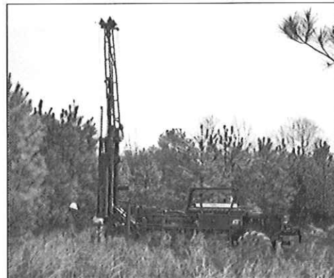
CTL's ATV can drill in rough terrain
