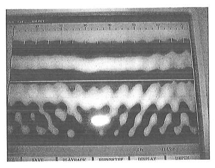
The GPR scanning at 25" deep in all areas inspected were consistant showing no large voids at this depth any where scanned at this inspection.
