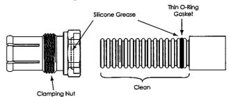
Step 4. Add clamping nut and cut cable. Push clamping nut on cable. Use twisting motion to assure spring contacts snap into groove. Refer to cutaway view in Step 6. Grip clamping nut with one hand and align edge with scribed line. Then carefully cut outer conductor and foam dielectric material flush with end of clamping nut, exposing center conductor. Make shallow cut; do not damage center conductor. Use hacksaw with fine-toothed blade or model maker's saw.
