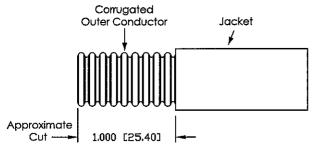
Step 2. Make second jacketing cut. Scribe line on ridge of exposed corrugated outer conductor. Line must be at least 13/32 in (10mm) from end of cable. Remove jacket to dimension shown using straight-edged piece of heavy paper wrapped around cable to guide cut.
