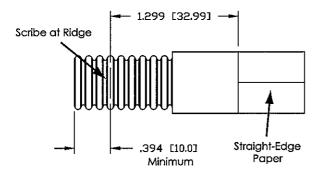
Step 3. Install gasket. Add thin O-ring gasket to second fully-exposed corrugation groove from jacket. Apply thin coating of silicone grease to outer surface of gasket and gasket lead chamfer in clamping nut using finger tip. Do not allow silicone grease on threads of clamping nut.
