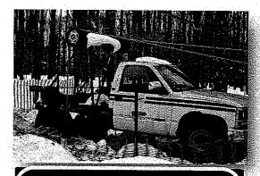
Although recently replaced with another surplus pick-up truck, this tow-system has been in use at Blackwater Falls sledding area for nearly 50 years. The DNR hopes to replace it with a new surface lift or tow system.
