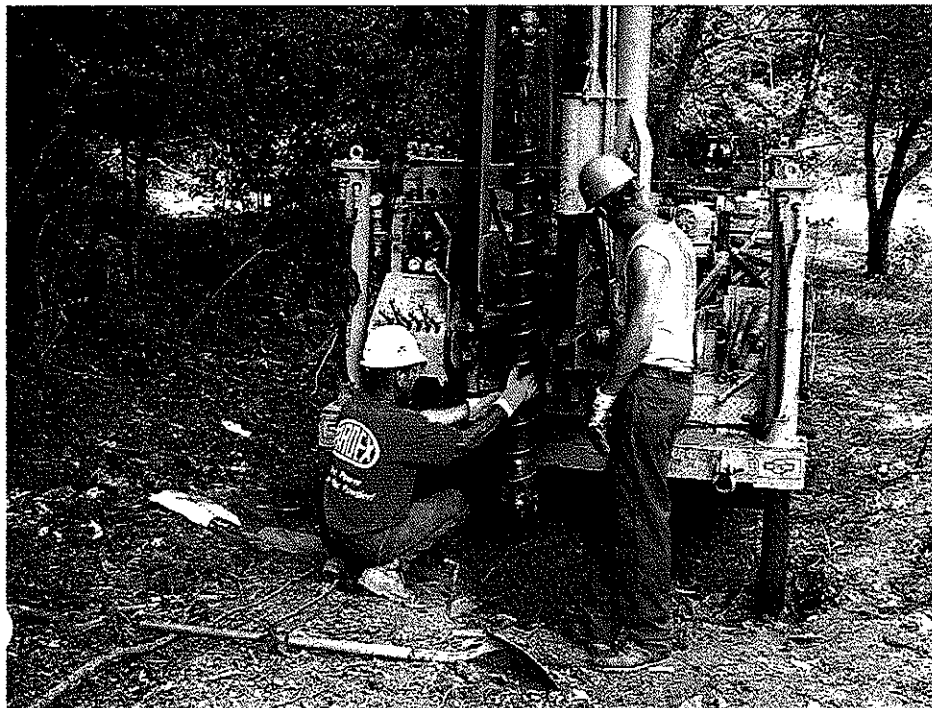
Drilling and sampling performed as part of the D'Appolonia field exploration program.
