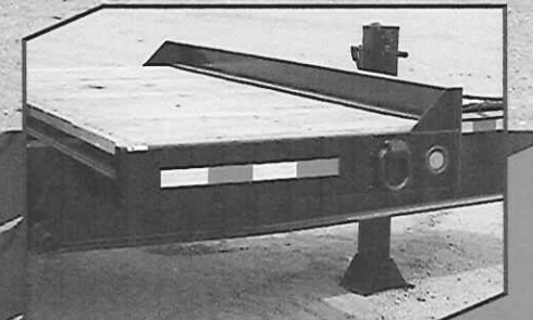
Standard 4-foot stationary deck gives room for longer equipment and makes towing easier.
