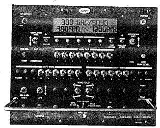
Standard bar control panel with computerized application rate control and spray controlled in 1' increments.
