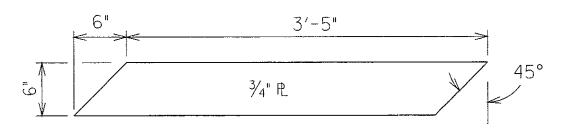
GALVANIZED 3/4" PLATE - MARK P2 (3 - Required) Rev. 09/08
