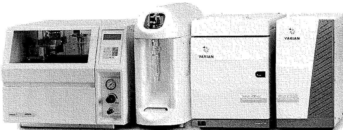
Soil/Drinking Water Analysis. Use the Archon™ AutoSampler Stratum PTC Purge and Trap concentrator with a Varian 431-GC and 210-MS for the measurement of Volatile Organic Compounds (VOCs) in drinking water, wastewater and soil
