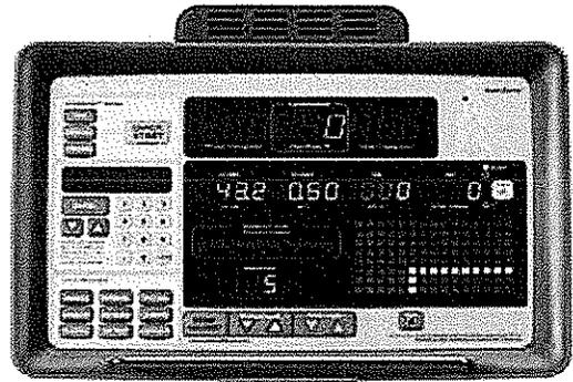
The E870 features an easy to operate dot matrix display with bright LED readouts. A numeric keypad makes entering workout data simple.
