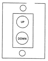
for "up/down" control of motorized hose reel, also available with rocker-switch.
