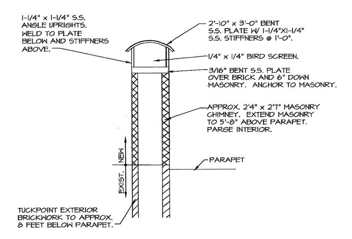
CHIMNEY REPAIR DETAIL
