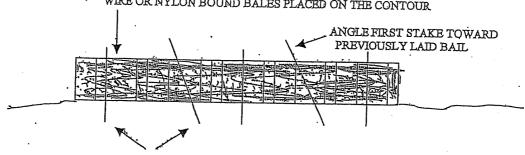
2 - 2 INCH X 2 INCH STAKES, 1 % FEET TO 2 FEET IN THE GROUND
