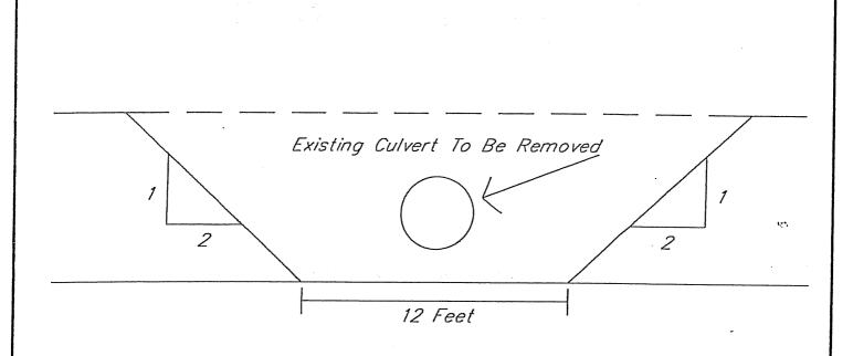
Drawing for Sediment Cells #3, #4, #5 Showing Typical Cut In Berm
