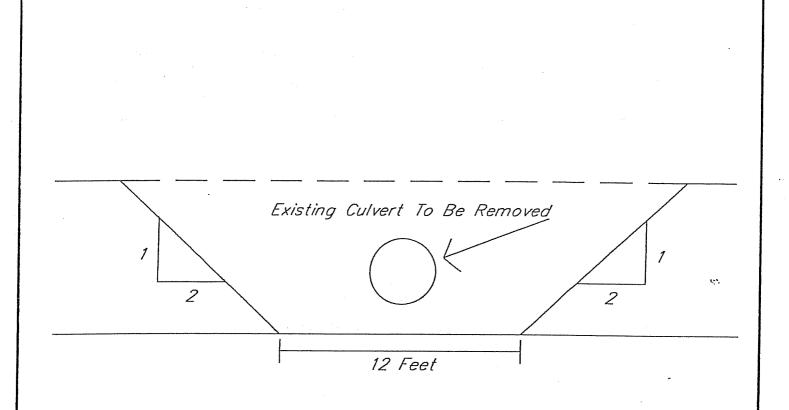
Drawing for Sediment Cells #3, #4, #5 Showing Typical Cut In Berm
