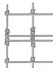
Note: Type Fw-4-5 Nicopress Dval Sleeve Wire Splices, or other equal sleeve splices approved by the Engineer, may be used in lieu of the above wrapped wire splices. TYPICAL WIRE FENCE SPLICE
