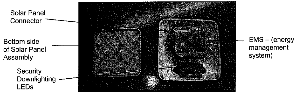
Figure 17: Head with the Solar Panel Assembly Removed
