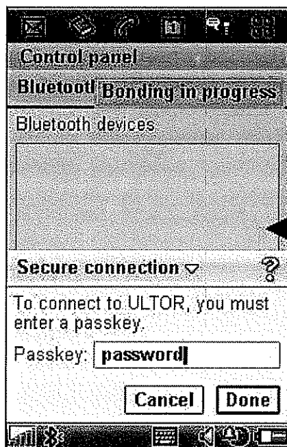
Figure 2 - Authentication example during the Bluetooth pairing process
