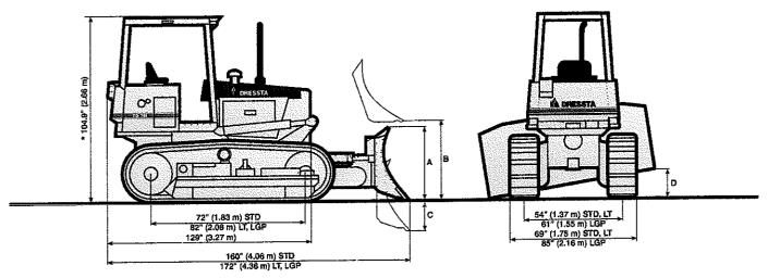
\* Overall height with Cab ROPS - 106.2" (2.70 m) Vertical dimensions include 2 11' (53 6 mm) grouser height
