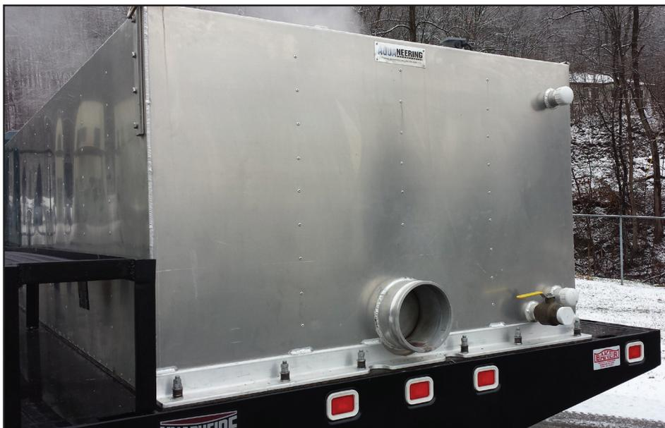
**The fish distribution tanks have a water capacity of approximately 1,200 gallons and contain five separate compartments for storing fish on their way to distribution.**
