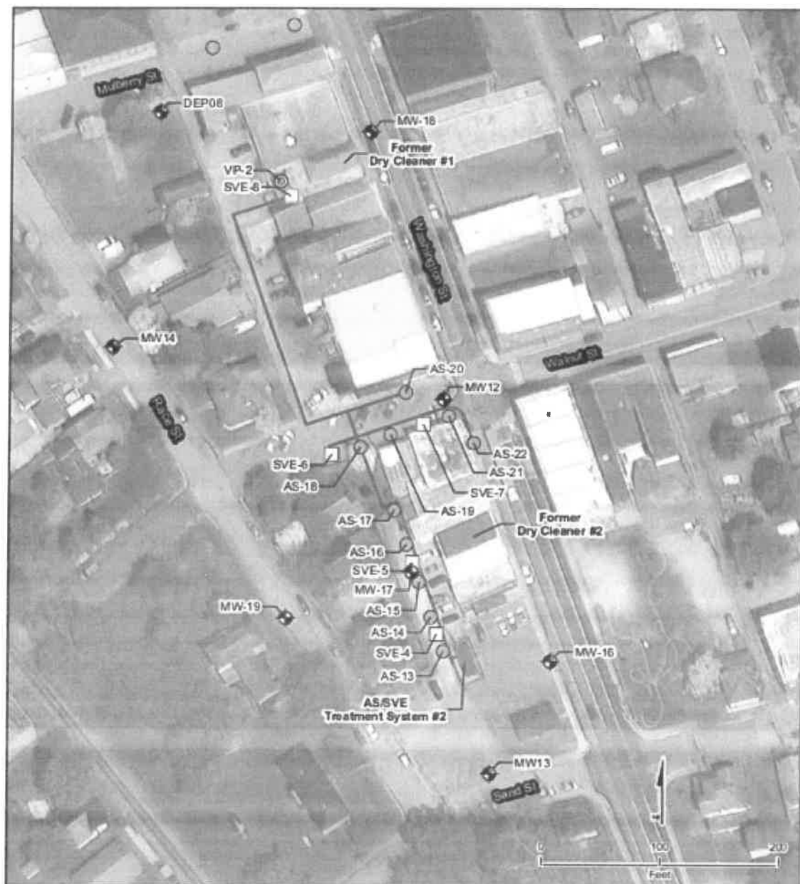
Figure 2: Configuration of Treatment System 2
