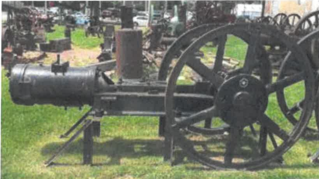
South Pin Half Breed Pump 18'-8" long, 4'-5" wide
