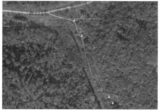
Triad proposes to accomplish the test borings with a track- or ATV-mounted rotary auger drill rig and perform Standard Penetration Testing in borings B-1 through B-4 and rock coring through the base of the mined-out coal seam in PZ-1 and PZ-2. Considering these two borings may encounter coal pillars, Triad proposes to drill up to two offset holes at each location to allow the inclinometer to be installed in the open void of the mined seam. The proposed drilling depths are as follows:
