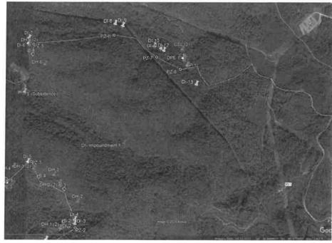
Triad proposes to accomplish the test borings with a track- or ATV-mounted rotary auger drill rig and perform Standard Penetration Testing in the borings and rock coring through the base of the mined-out coal seam in PZ-1 through PZ-8. Considering these borings may encounter coal pillars, Triad proposes to drill up to two offset holes at each location to allow the piezometer to be installed in the open void of the mined seam. The proposed drilling depths are as follows:
