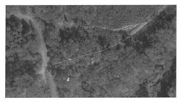
Triad proposes to accomplish the test borings with a track- or ATV-mounted rotary auger drill rig and perform Standard Penetration Testing and rock coring through the base of the mined-out coal seam. Considering boring may encounter coal pillars, Triad proposes to drill up to two offset holes at each location to allow the piezometer to be installed in the open void of the mined seam. The proposed drilling depths are as follows:
