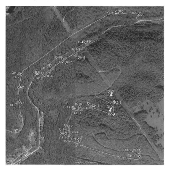
Triad proposes to accomplish the test borings with a track- or ATV-mounted rotary auger drill rig and perform Standard Penetration Testing in the borings and rock coring through the base of the mined-out coal seam in PZ-1 through PZ-5. Considering these borings may encounter coal pillars, Triad proposes to drill up to two offset holes at each location to allow the piezometer to be installed in the open void of the mined seam. The proposed drilling depths are as follows:
