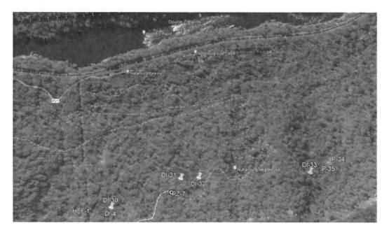
Triad proposes to accomplish the test borings with a track- or ATV-mounted rotary auger drill rig and perform Standard Penetration Testing and rock coring through the base of the mined-out coal seam in borings PZ-1 through PZ-7. Considering these seven borings may encounter coal pillars, Triad proposes to drill up to two offset holes at each location to allow the piezometer to be installed in the open void of the mined seam. The proposed drilling depths are as follows:
