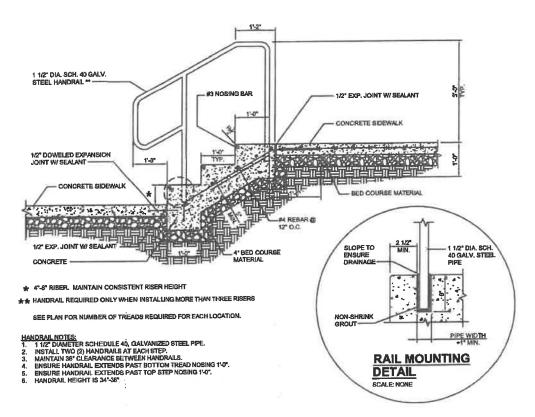
CONCRETE STEP & HANDRAIL DETAIL
