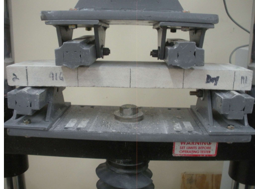
Photo No. 10 ASTM C880 – Specimen Loading Detail
