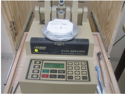
Photo No. 13 ASTM C1353 – Test Apparatus (Depicted with Pre-Abrasion Test Specimen)
