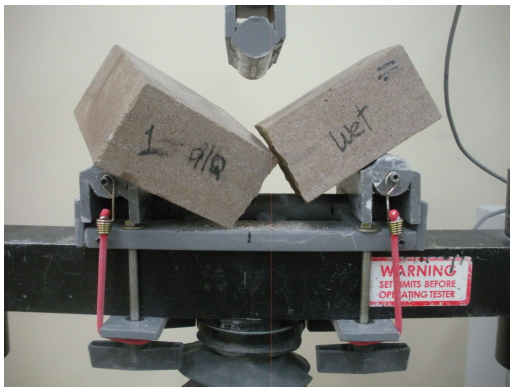
Photo No. 7 ASTM C99 – Representative Perpendicular to Rift Loading Specimen Failure Mode
