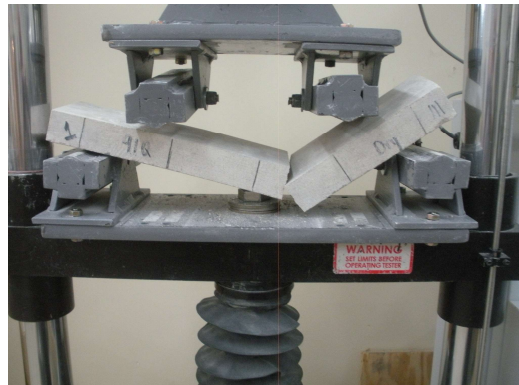
Photo No. 12 ASTM C880 – Representative Parallel to Rift Loading Specimen Failure Mode
