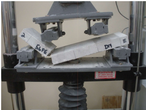
Photo No. 11 ASTM C880 – Representative Perpendicular to Rift Loading Specimen Failure Mode
