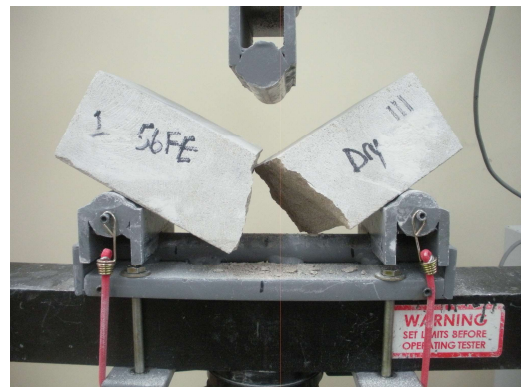
Photo No. 8 ASTM C99 – Representative Parallel to Rift Loading Specimen Failure Mode
