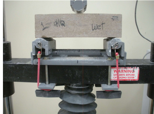
Photo No. 6 ASTM C99 – Specimen Loading Detail
