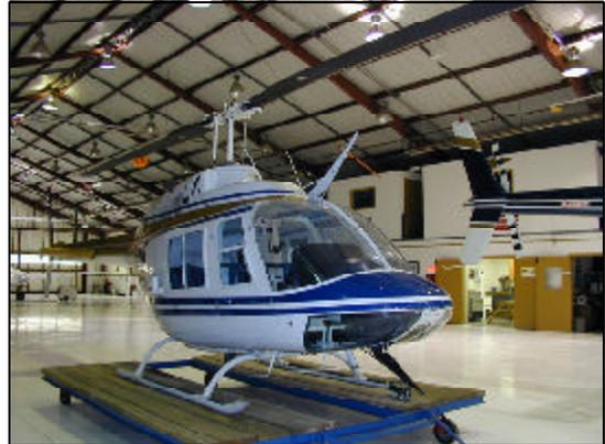
The specifications for the helicopter included an airframe 11720 TT, engine 10701 TT, low skid gear, particle separator, wire strike protection, aircom bleed air heater with defroster, rotor brakes, dual controls, and 1,200 pound cargo hook.
