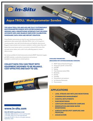
Acquired from the vendor In-Situ, DEP's new Aqua TROLL 600 sondes can provide data from a variety of aquatic locations including lakes, streams, wetlands, stormwater, dam monitoring, groundwater, mine water, and more. Using these devices, DEP can evaluate water quality with data such as actual and specific conductivity, pH/oxidation/reduction potential, salinity, total dissolved solids, resistivity, density, turbidity, temperature and pressure, ion selective electrodes, and fluorometers.
