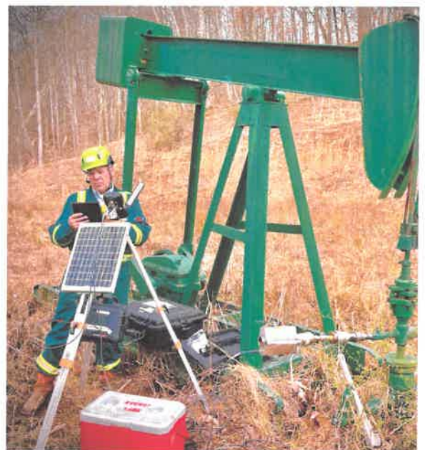
Curtis Shuck, QMS measuring methane at a marginal well for Antero Resources in Doddridge County, WV.
