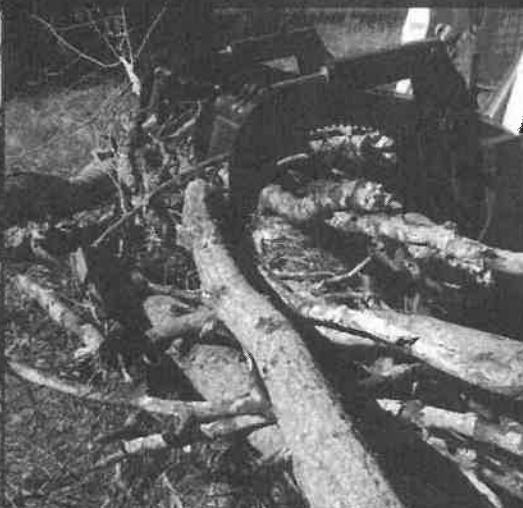
BUCKET CONSTRUCTED OF 1/2" THICK GRADE 50 STEEL
