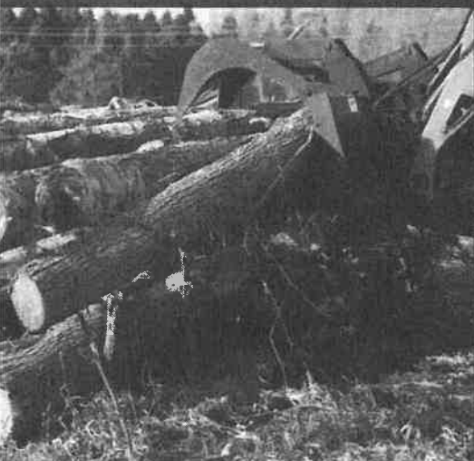
REINFORCED TUBING FOR ADDED TINE STRENGTH
