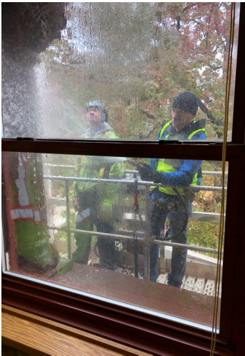
SGH performed water testing at second floor windows.
