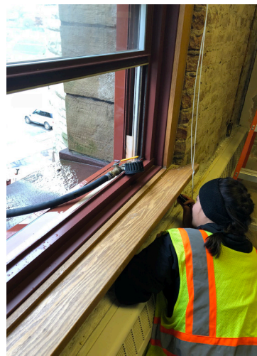
SGH performed water testing at second floor windows.
