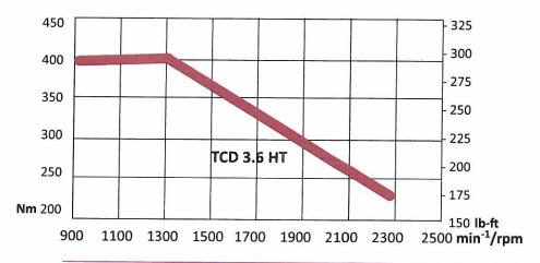
The steep torque curve makes the engine act in a way that makes the roller strong also in hilly conditions
