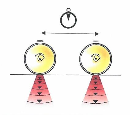
A small time difference in start-up makes vibration reach correct frequency very fast
