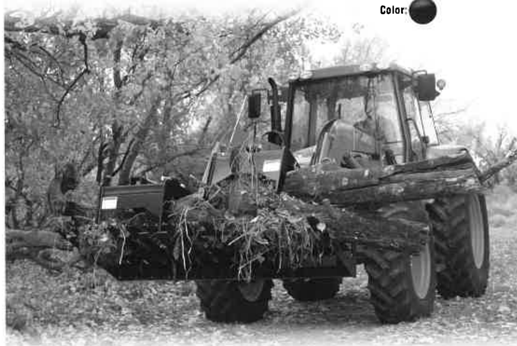
Open ends allow for greater capacity.
