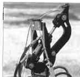
Optional Hydraulic Wing Unlock allows user to unlock the wings from the tractor seat.
