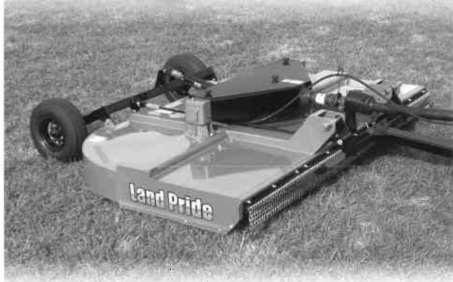
Narrow tongue on pull-type allows for tight turns
