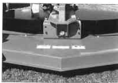
Low deck pivot allows for greater side to side flotation on the wing decks.
