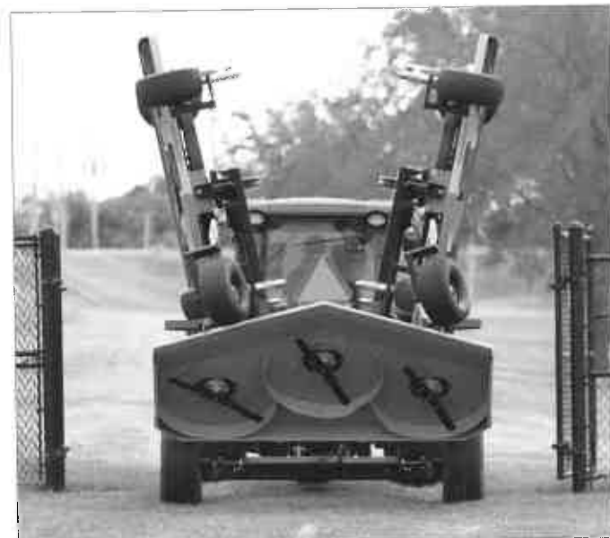
Transport width of 9'6" allows for safe transport from site to site.
