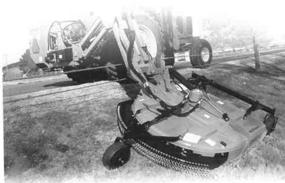
Optional gauge wheel deck allows the cutter to float over undulations without having to constantly monitor terrain conditions.
