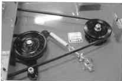
Over center release easily takes tension off the drive belts during extended off time, or for belt replacement.
