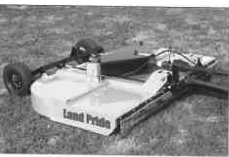
Narrow tongue on pull-type allows for tight turns.
