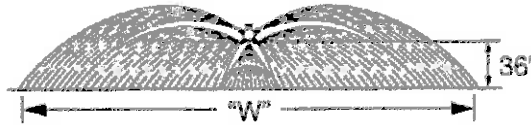
W = Maximum effective coverage with nozzle mounted at 36" height.
