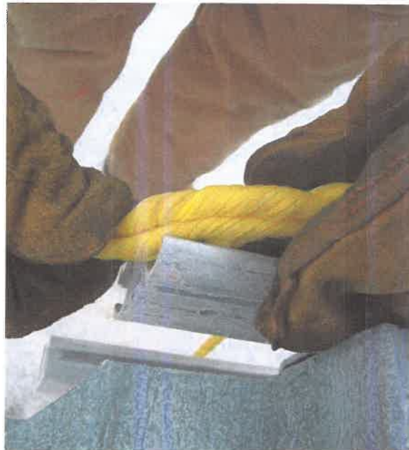
Right Below: Flattening the rope to pull ends out to the side of the Extrusion channel
