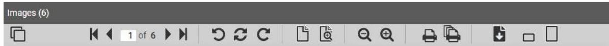
Figure 4-123: SMART Image Viewer Tool Bar. SMI's Image Viewer allows users to rotate the image, reload the image, decrease or increase the size of the image, move the image down, and print one image or all images for the work item.
