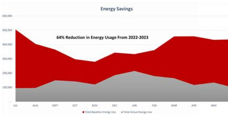
**ABOVE:** ZDS designed and implemented a geothermal system for *Riverside High School in Kanawha County* showing a **reduction in energy use of over 64% with an EUI of 30.6 from an EUI of 84.**
