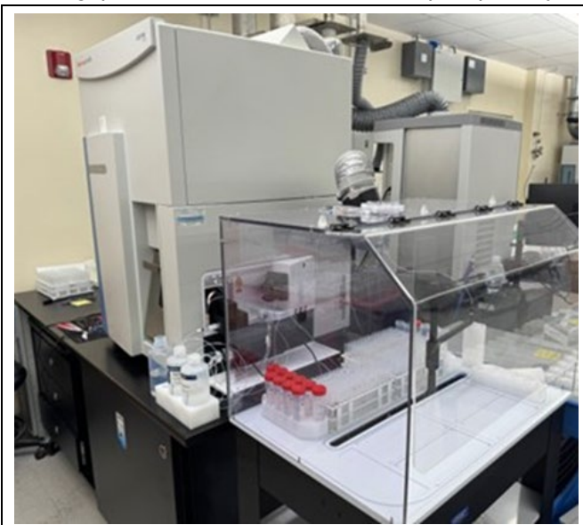
Exhibit 23. 1 of 3 ICPMS that RTI Will Use to Analyze Water Samples with Method 200.8
