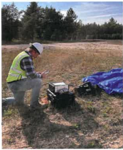
FIGURE 2-8: PARSONS BIL-QMS PERFORMING METHANE LEAK QUANTIFICATION FROM AN ORPHANED WELL CASING CUTOFF AT SURFACE
