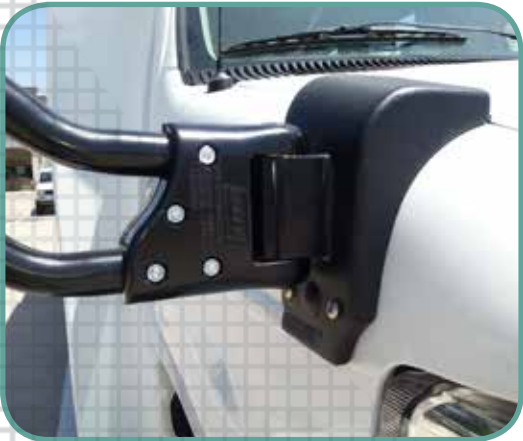
Fender Mount Rearview Mirror Assembly with Spring-Break® Detent (Non Combination Assembly)
