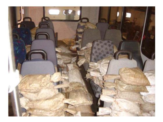
DIAL INDICATORS IN POSITION BUS LOADED TO 2.5 TIMES GVL (10,725 LBS)
