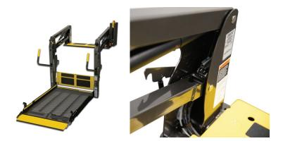
The NCL1000-2 Century Series also features new and improved inboard barriers, baseplates, vertical channels, and lower parallel arms for a more rigid and stable ride.
