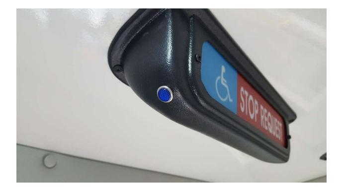
The ADA Occupant Stop Request Lights the Blue Side of the Sign and Signals Driver of an ADA Stop Request via Touch Tape Switches.
