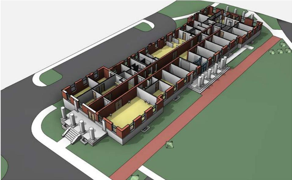
3D models (left and below) helped PWVG's team plan locations for vertical risers for new MEP systems, and a new elevator shaft in the historic building to limit architectural interventions.
