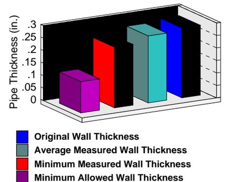
**Comments:** Testing at the return side pipe again shows dramatically higher and more uniform wall thickness due to lower corrosion activity; with no obvious explanation to such occurrence. Extremely long service life remains.
